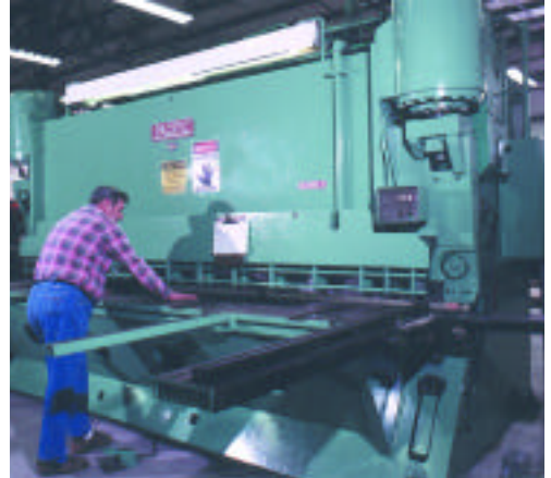
One-half inch x 12 ft. shear at Windsor, Connecticut service center supplies customers in the northeast with sheet and light plate, cut-to-size.
