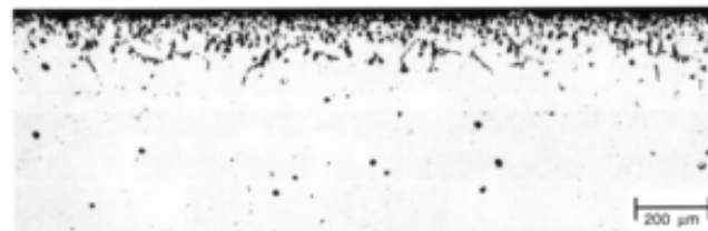
RA330 alloy Average Metal Affected = 8.7 Mils (221 \mu\text{m} )
