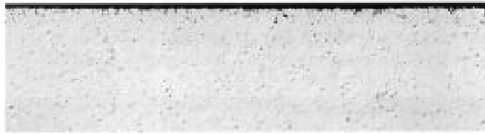
HAYNES 556 alloy Average Metal Affected = 1.1 mils (20 µm)
